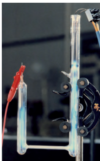
Figure 7: Krypton lamp according to Engelhard for the realization of the unit of length 1960–1983.
