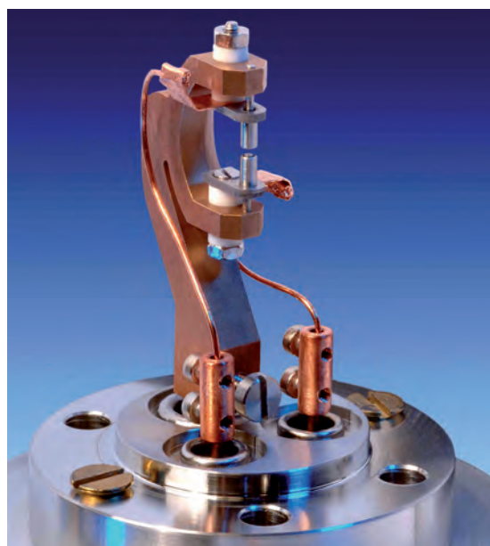
Figure 14: On the left: Vacuum recipient with ion trap (in the centre) for the spectroscopy of single ytterbium ions [41]; on the right: Detail of the latest trap arrangement, a so-called end cap trap which has been used since the beginning of 2010.
