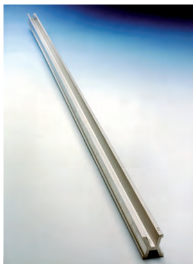
Figure 6: International prototype of the meter, a line standard with X-shaped cross-sectional profile made of platinum-iridium.
