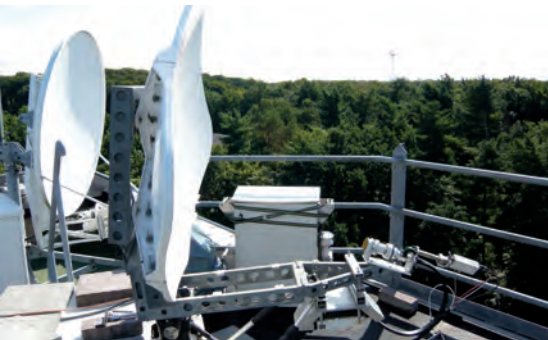
Figure 12: Establishment of a transportable satellite terminal for calibration of the time comparisons via TWSTFT with the stationary facility (background).
