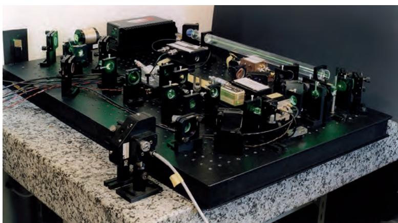
Figure 11: I_2 -stabilized, frequency-doubled Nd:YAG laser.
