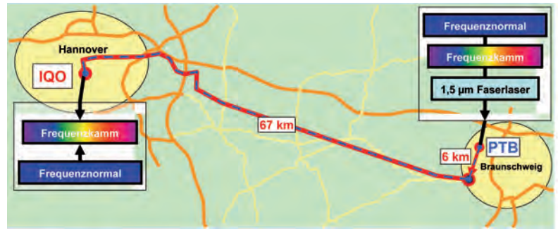
Figure 19: Scheme of a comparison of optical frequency standards via a commercial optical fiber connection (blue and red lines). At PTB, a fiber laser is stabilized to an optical frequency standard at a wavelength of 1.5 \mu\text{m} . Its radiation is transferred by means of optical fibers to Leibniz University in Hanover where it is compared with the frequency of a frequency standard with cold magnesium atoms [79].
