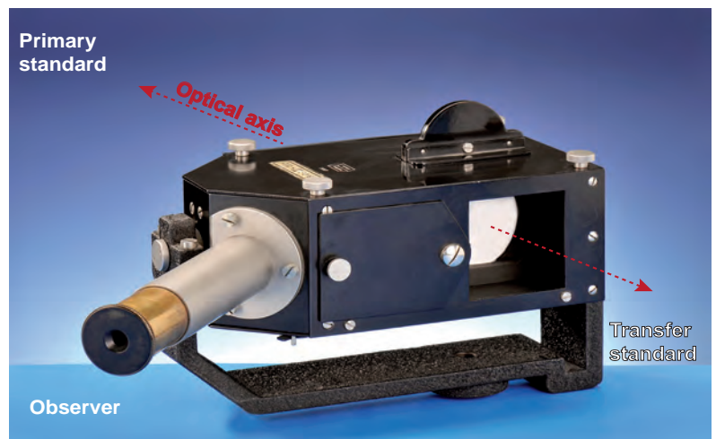
Figure 2: Lummer-Brodhun contrast photometer.
