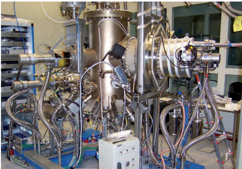
Figure 4: PTB's Molecular Beam Epitaxy (MBE) facility for the production of GaAs layer crystals for quantum Hall resistors.
